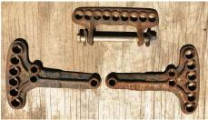
**Above**: Identification complete! The various parts of a clevis hitch. Photo by Jeff Kaskey **Below:** An illustration of a walking plow with a complete clevis hitch.
